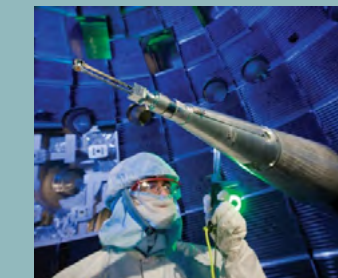
Modern-day stockpile stewardship depends on experiments, historic test data, and high-performance computing to ensure the long-term viability of the U.S. deterrent without additional underground nuclear tests. Left: Before each NIF experiment, a technician uses a positioner to precisely center the target inside the chamber. The positioner serves as a reference to align the laser beams. Right: This simulation shows hydrodynamic instability of two fluids mixing in a spherical geometry. Such simulations provide valuable data sets for understanding turbulence models important to ICF and stockpile stewardship applications.
